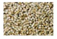
first, the sawdust generally comes from seasoned wood, so already has a lower moisture content than freshly harvested wood and needs less (or no) drying. The main advantage over other wood fuels is their energy density ( $H_d \approx 5 \ kWh / kg$ ,  $3100 \ kWh/m^3$ ). Price of that fuel is different from place to place, but on world market can be found as  $200 \ Eu / t$ . Because in Montenegro exists a few wood
