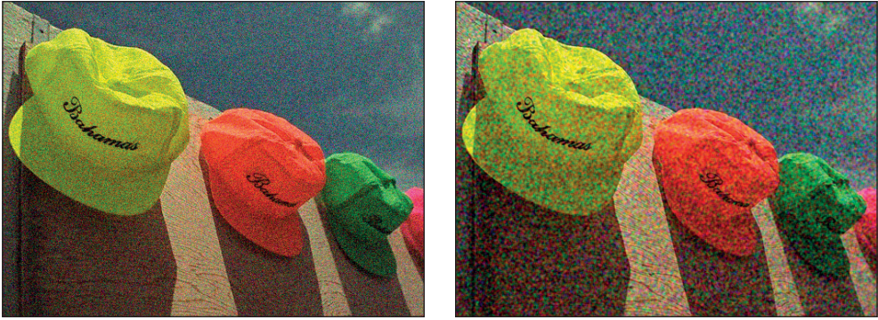
Fig. 8. Color test image fragments corrupted by AWGN (left) and spatially correlated (right) noise having the same variance equal to 130
