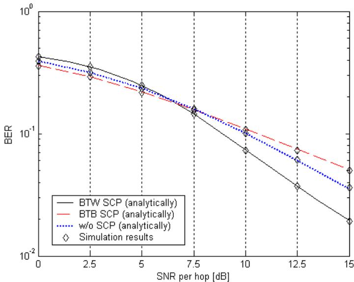
Figure 3. BER of DPSK modulated OFDM AF relay system with SCP
