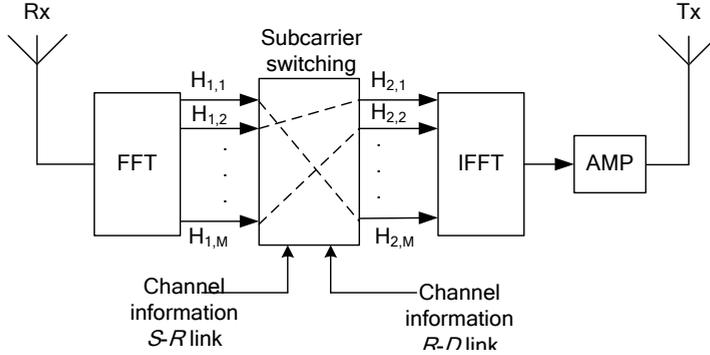
Figure 2. Block scheme of the OFDM-based fixed gain relay terminal with SCP
