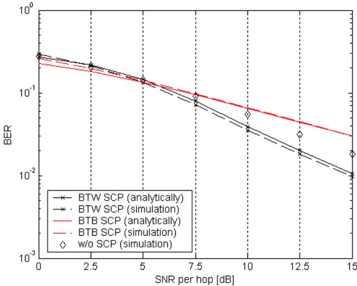
Figure 4. BER of BPSK modulated OFDM AF relay system with SCP
