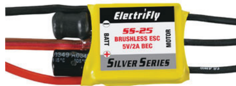
Sl. 3. Invertor napona (Speed Control SS-25)
