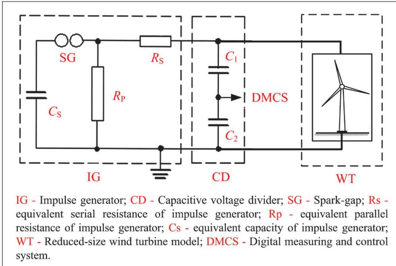
Figure 4. Measuring and control system in the high-voltage laboratory
