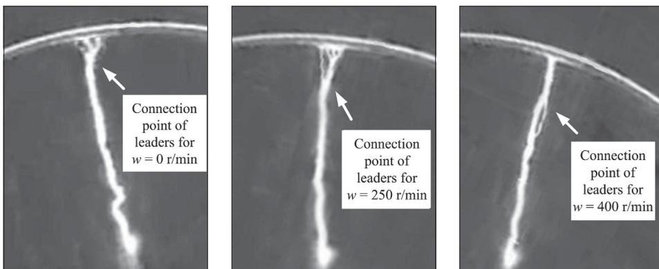
Figure 5. Enlarged photos of typical leaders connection
