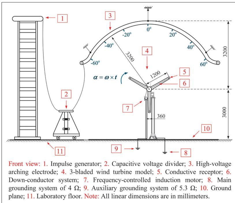
Figure 1. Experimental setup for reduced-size wind turbine model testing
