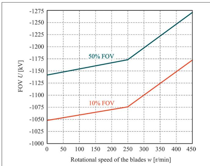
Figure 8. Impact of blade rotation on the 50% and 10% FOV
