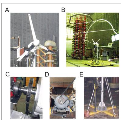
Figure 2. (A) Three-bladed wind turbine rotor with the conductive receptors at the blade tips; (B) Arching electrode set above the wind turbine model; (C) Main shaft ball bearings; (D) 4 kW frequency-controlled induction motor with belt coupling; (E) Cross-like base
