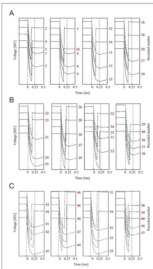
Figure 7. Characteristic waveforms when a negative impulse voltage is applied to the arching electrode. (A)  $w = 0$  r/min; (B)  $w = 250$  r/min; (C)  $w = 400$  r/min
