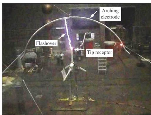
Figure 3. Photo from the control room when a negative impulse voltage is applied to the arching electrode
