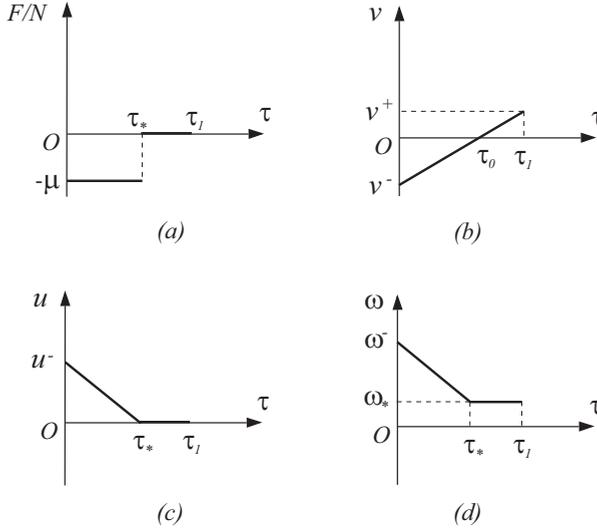
Figure 2: The variation of the force ratio ( $F/N$ ), the velocity components of the contact point ( $u$  and  $v$ ), and the angular velocity ( $\omega$ ) during the impact, in the case  $\tau_* < \tau_1$ , where  $\tau_*$  is defined by  $u(\tau_*) = 0$ .
