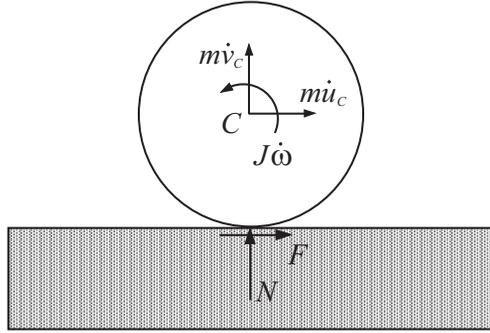
Figure 1: A spinning circular disk during an impact with a fixed horizontal surface. The reactive forces from the rough surface are  $N$  and  $F$ , the angular acceleration of the disk is  $\dot{\omega}$ , and the acceleration components of its mass center are  $\dot{u}_C$  and  $\dot{v}_C$ .
