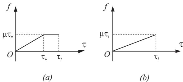
Figure 4: Routh's impact diagram showing the variation of the tangential impulse  $f$  vs. the normal impulse  $\tau$ , in the case  $u^- < 0$ : (a)  $\tau_* < \tau_1$ ; (b)  $\tau_* > \tau_1$ .
