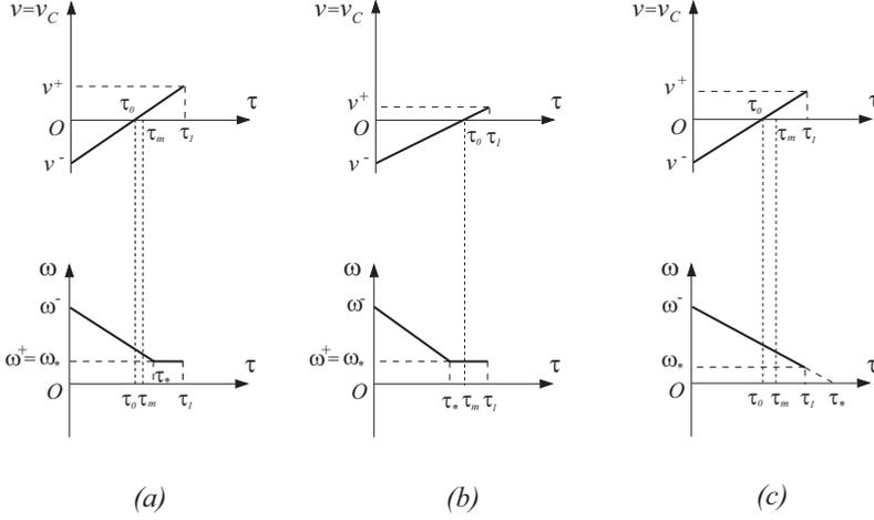
Figure 5: The kinetic energy attains its minimum during (a) the sliding phase of the impact if  $|u^-/v^-| > \zeta\mu$ , and in that case  $\tau_0 < \tau_m < \tau_* < \tau_1$ ; (b) the rolling phase of the impact if  $|u^-/v^-| < \zeta\mu$ , and in that case  $\tau_* < \tau_m = \tau_0 < \tau_1$ ; (c) after the end of the compression phase, in the case of sliding throughout the impact.
