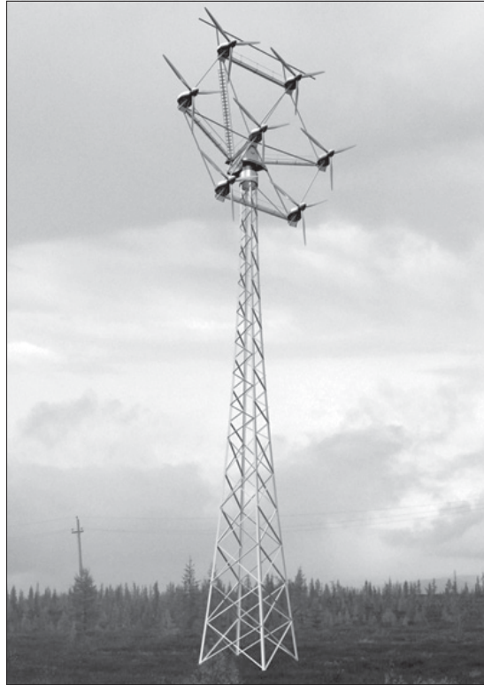
Figure 2. Module wind turbine unit with total capacity of 52.5 kW
